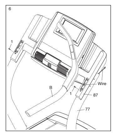
Set the right handrail assembly (B) onto the right Upright (77). Make sure that no wires are pinched. Attach the right handrail assembly with two 3/8" x 5 1/2" Screws (5) and two 3/8" Star Washers (8). Note: Start the lower Screw first.
